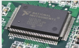
Single-chip IEEE 488.2 Talker/Listener interface to the GPIB
