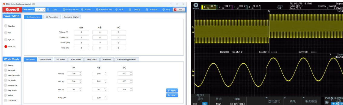
Fig. 4-4 AC+DC @150V/50Hz, superimposed with 100Vdc, trigger @0°
