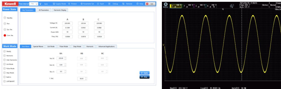
Fig. 4-3 Sine wave mode, single phase @220V
