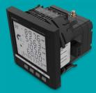
AXM-WEB2 includes dual Ethernet ports and Wi-Fi communication channel for the Acuvim II and Acuvim-L Series power meters. Multi-protocols are supported such as IEC61850 2nd Ed., Modbus, MQTT, Google IoT, BACnet, and DNP3 V2.
