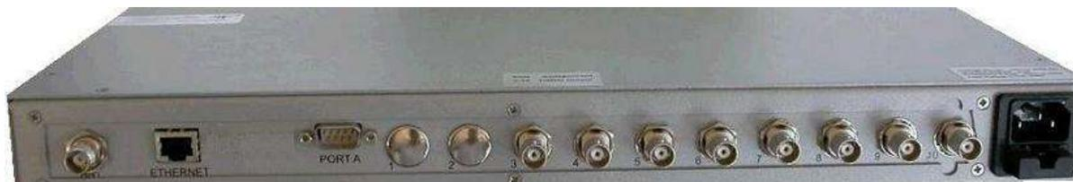
Dependent upon the configuration, a full width module may be used in place of a half width module. Connections for Ethernet, RS232, and GNS antenna should be made as described above.
