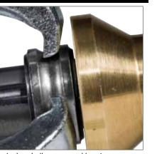
Lock on ball grooves and bearing races
