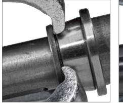
Tapered roller bearing on shaft
