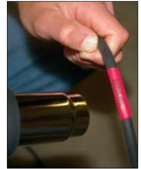
3 Use Heat Gun To Shrink Material Around Object
